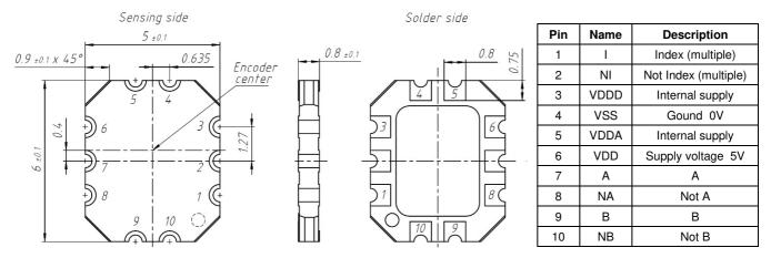
Fig. 3 Encoder dimensions (mm) and pin-out. "Encoder center" must be centered with respect to Readout Radius (see Fig. 4).
