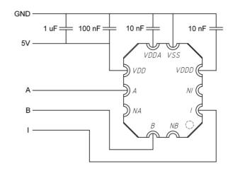
Fig. 5 Recommended schematic. The supply filter capacitor should be  $1\mu F$  or more. The capacitors 100nF and 2 x 10nF should be placed close to the device. Connections A, B and I are required for programming and linearization.
