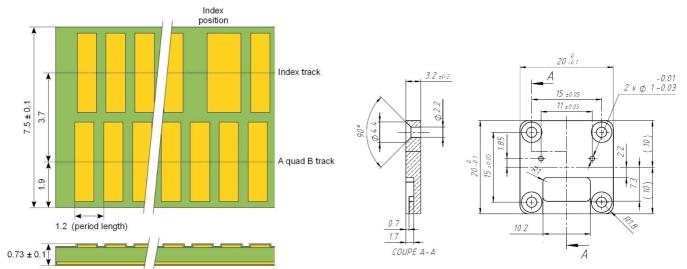
Fig. 4 Linear scale with period length 1.2 mm (drawing not to scale).
