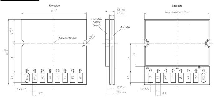
Fig. 3 Dimensions of IT3402 encoder on encoder-holder type B. The "Encoder center" must be centered with respect to the width of the linear scale (Fig 4).
